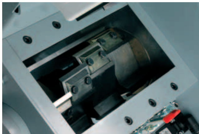
Staggered blades to guarantee accurate and clean cutting action
